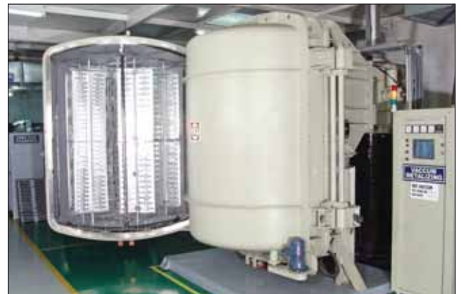
Vacuum Metalizing Chamber
