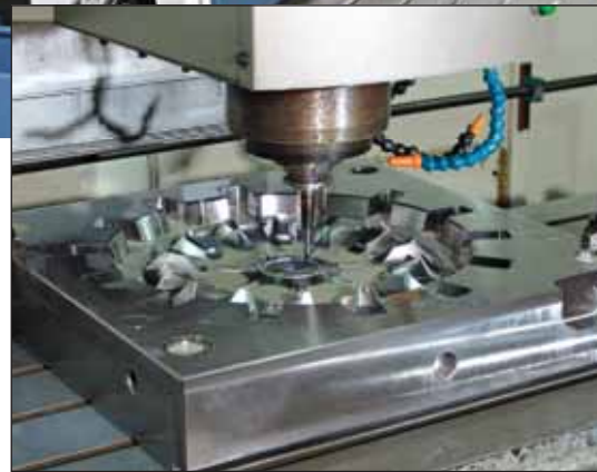
CNC machining for Wheel Cover Cavity
