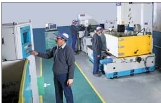
Electrical Discharge Machines
