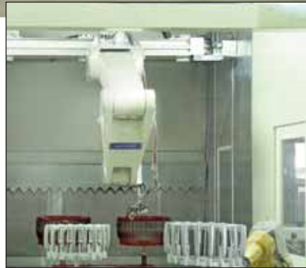
3 Coat Rotary spindle robotic paint line
